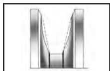
Worn Groove Sidewalls
